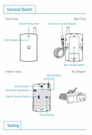
Connect the adaptor with the connector and then plug the adaptor into wall socket. The detector enters normal working mode after the LED indicator flashes once. Knocking glass object (e.g. knocking a glass bottle with a metal spoon), the detector receives the high voice frequency signal. Meanwhile, the LED indicator flashes once which means the detector works properly.
