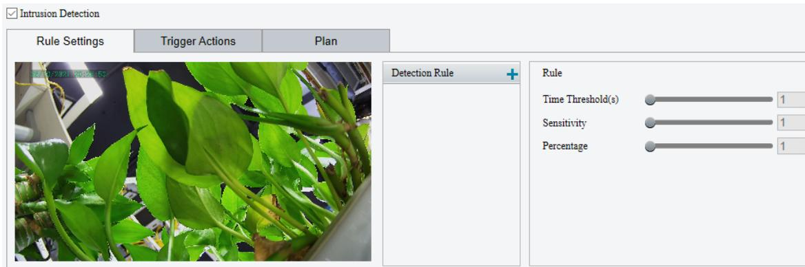
1. Select the **Intrusion Detection** check box to enable intrusion detection.
