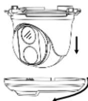
3. Connect the cable and then secure the dome.
