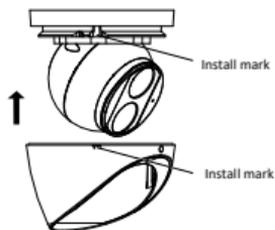
5. Adjust the monitoring direction. Adjust the monitoring direction, then tighten the screw.
