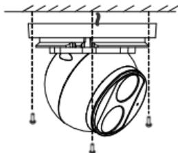
4. Mount your camera. Mount the housing with install mark aligned.
