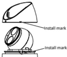
3. Install the base plate and the camera. Connect cable and protect it with waterproof tape and attach dome to ceiling with taping screws.
