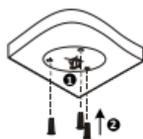
2. Remove the bottom ring, turn bottom ring anticlockwise to loosen it.
