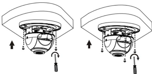
5. Adjust the monitoring direction of the lens (tighten screws after vertically adjusting the lens). The lens can horizontally turn by rotating the lens base, as shown by ❶ in the following figure. After loosening the fastening screws, you can vertically turn the lens, as shown by ❷ in the following figure.
