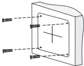
4. Mount your camera onto the wall. Lead tapping screws through the guide holes in the camera base and fix them on the wall using a screwdriver.
