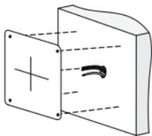
2. Drill holes on the wall. Use a  $\phi$  6-6.5mm drill bit to drill 30mm-depth guide holes according to the positions marked by the sticker.
