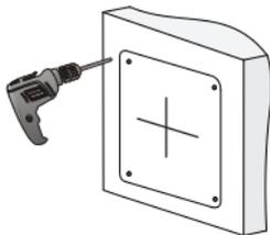
3. Mount the plastic rivets of self-tapping screws. Knock the plastic rivets into the guide holes and ensure that they are tightened up.
