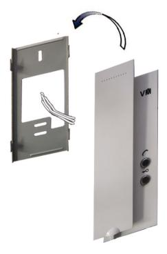
Carefully place the door monitor against the bracket and gently push down the monitor so that the pins on the bracket engage in the slots on the rear of the monitor.
