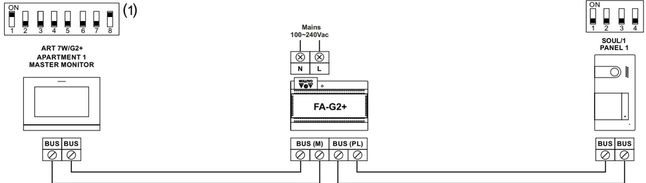
(1) Note: The monitor is set at the factory as **master** monitor.
