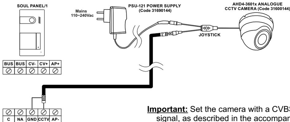
**Important:** Set the camera with a CVBS analogue signal, as described in the accompanying AHD4-3601x camera manual.
