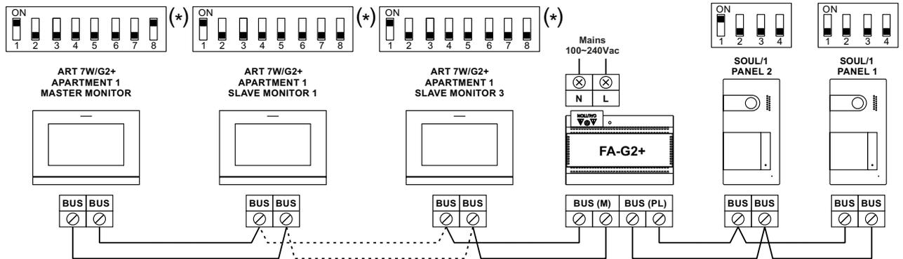
One apartment with two access panels and up to four monitors in distribution
