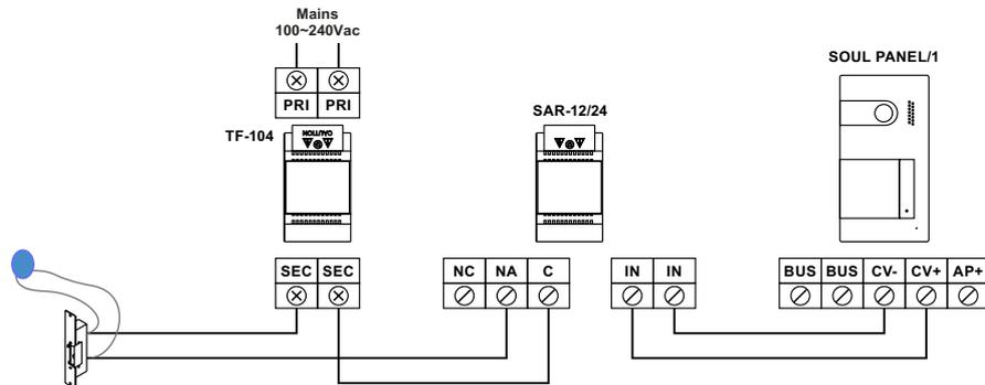
Connection of an auxiliary device at the relay output
