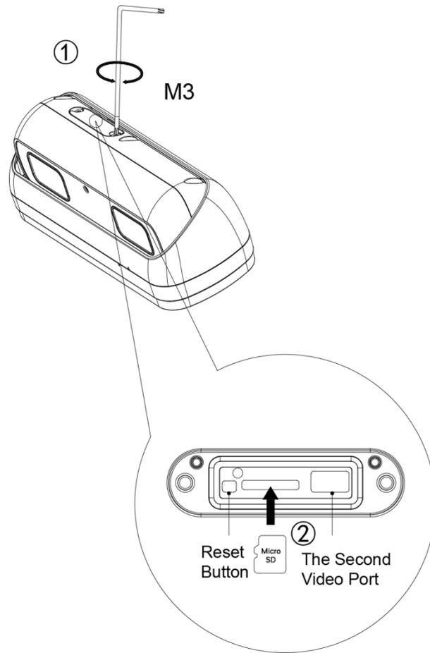
Press the reset button for 10 seconds to reset the device.
