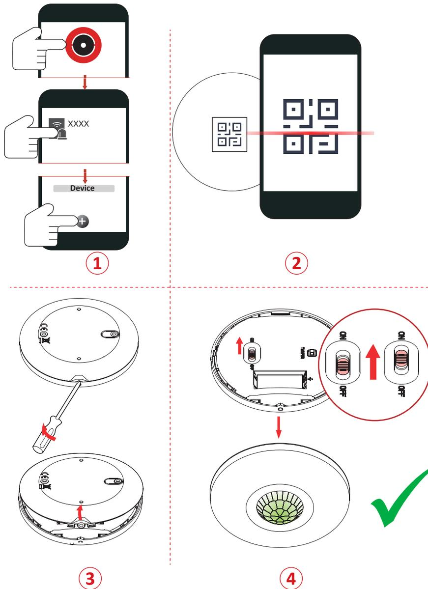
Note: Hold the tamper button, and make the device power off and then power on for re-enrollment.
