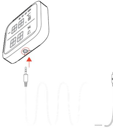
**Note:** The humidity detection will be disabled when using probe.
