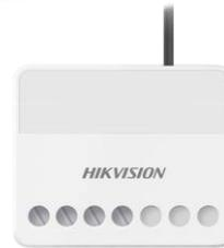
DS-PM1-O1H-WB Wall Switch is a device to control electrical power supply remotely. The device can directly connect to 100~240VAC source and open/close circuit manually via APP/Keypad/Keyfob or automatically by linking to different system events.
