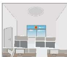
Light OFF when ambient brightness becomes higher than the preset lux level.
