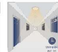
After holdtime, sensor dims light to standby dimming level for standby period.
