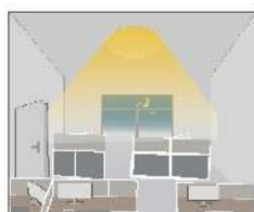
When ambient brightness is over than preset lux level, sensor will turn on light automatically
