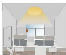
When ambient brightness is over than preset lux level, sensor will turn on light automatically
