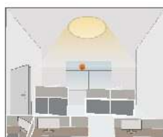
When ambient brightness is over than preset lux level, sensor will turn on light automatically
