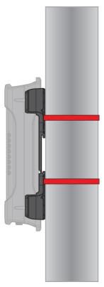
Figure 9 - Pole mount using DIN rail bracket
