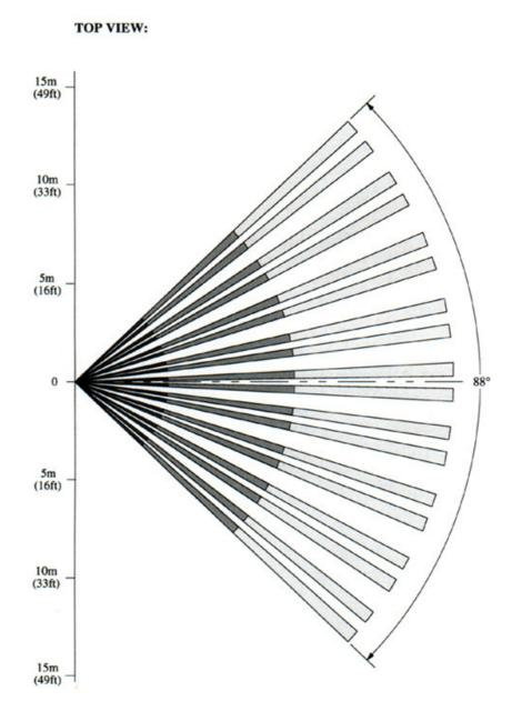
Figure 9 – detection pattern in the optimal temperature environment
