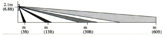
Figure 8 – side view, detection pattern in optimal temperature environment
